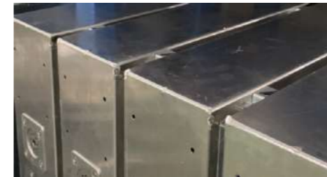
铝机箱焊接 Welding of aluminum case
