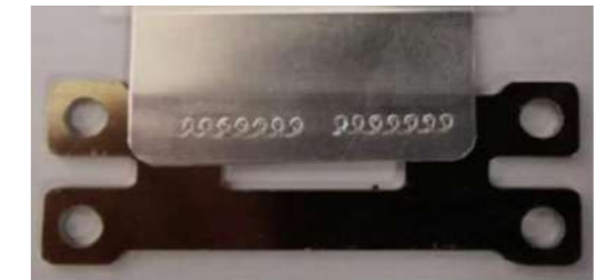
汇流排焊接 Bus bar welding
